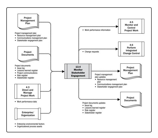
Figure 13-10. Monitor Stakeholder Engagement: Data Flow Diagram
