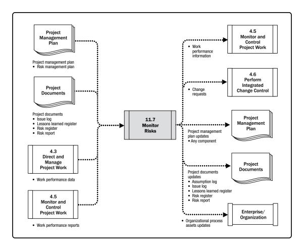
Figure 11-21. Monitor Risks: Data Flow Diagram
