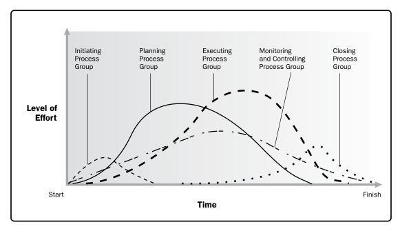
Figure 1-5. Example of Process Group Interactions Within a Project or Phase
