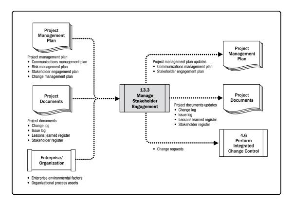
Figure 13-8. Manage Stakeholder Engagement: Data Flow Diagram
