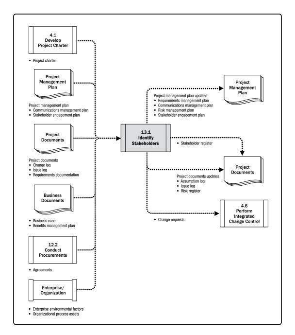
Figure 13-3. Identify Stakeholders: Data Flow Diagram
