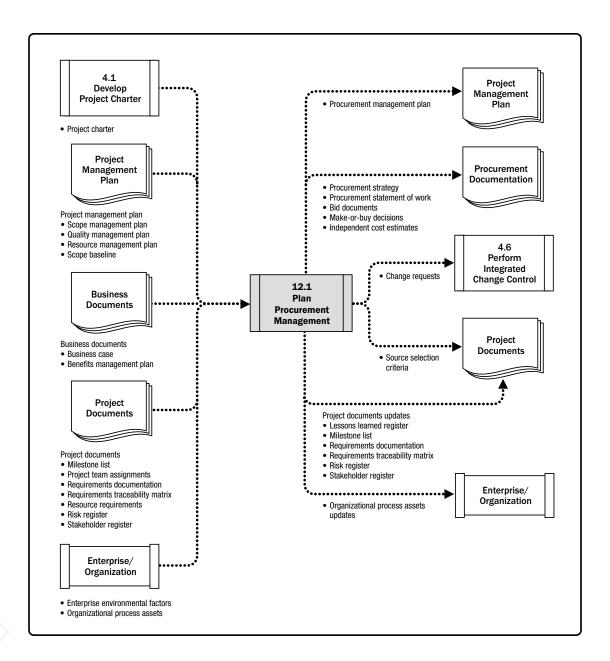
Figure 12-3. Plan Procurement Management: Data Flow Diagram
